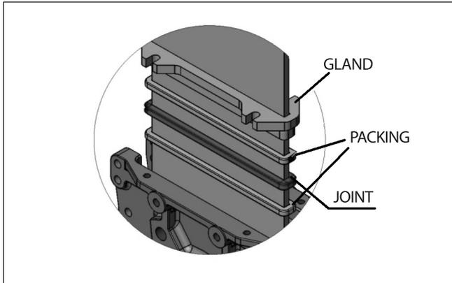
**SYNTHETIC + PTFE:** This packing is composed of braided synthetic fibres soaked in PTFE both inside and out. It is for general use in hydraulic applications in both pumps and valves and in all types of fluids, especially corrosive ones, including concentrated and oxidising oils. It is also used in liquids with solid particles in suspension.
