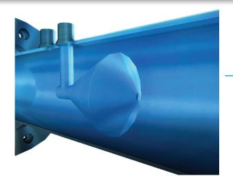
Centrally-located cone directs flow to the outside wall effectively conditioning disrupted flows.
