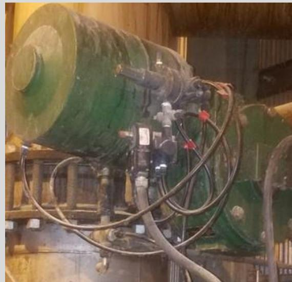
*Complex ad-hoc piping and integration with various components to achieve fail-safe with external air reservoir.*
