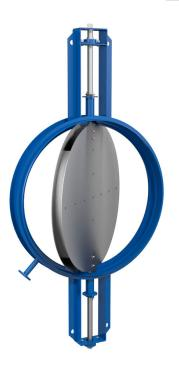
Flanged or wafer butterfly damper valve. Cast or welded body and disc depending the diameter of the valve. Manufactured with different kinds of tightness depending the customer requirements (100% tight, 99,5% tight o 98,5% tight). Fabrication materials: S275JR carbon steel, HII carbon steel, 16MO3 carbon steel, different stainless steel qualities (aisi 304, 316, 310 ...). Depending the application.
