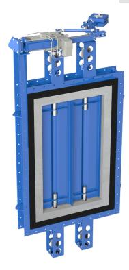
Flanged light butterfly, square, rectangular louvred type, several blades.. Welded construction body and disc. Manufactured with different kinds of tightness depending the customer requirements (100% tight, 99,5% tight o 98,5% tight). Fabrication materials: S275JR carbon steel, HII carbon steel, 16MO3 carbon steel, different stainless steel qualities (aisi 304, 316, 310 ...).
