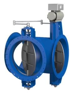
Flanged or wafer butterfly damper valve. Cast or welded body and disc depending the diameter of the valve. Manufactured with different kinds of tightness depending the customer requirements (100% tight, 99,5% tight o 98,5% tight). Fabrication materials: S275JR carbon steel, HII carbon steel, 16MO3 carbon steel, different stainless steel qualities (aisi 304, 316, 310 ...). Depending the application.
