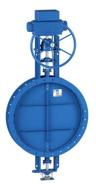
Flanged or wafer butterfly damper valve. Cast or welded body and disc depending the diameter of the valve. Manufactured with different kinds of tightness depending the customer requirements (100% tight, 99,5% tight o 98,5% tight). Fabrication materials: S275JR carbon steel, HII carbon steel, 16MO3 carbon steel, different stainless steel qualities (aisi 304, 316, 310 ...). Depending the application.
