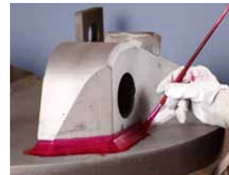
Dye penetrant test
